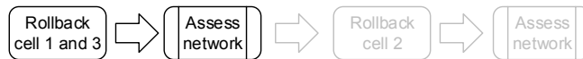
(b) The resulting sequence of corrective actions after the elimination of the collisions. The configurations of cell 1 and 3 are rolled back whereas the changes at cell 2 are accepted.
