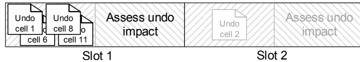
Figure 6.7: Correction window slot allocation. The order is defined by the variable assignment process from the previous step.
