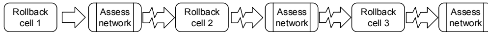
Figure 3.7: Adding constraints to a corrective action plan may result in the inability of processing all rollback actions. Due to the constraint |\mathcal{P}^{C^\perp}| < 2 , it is impossible to process all actions.
