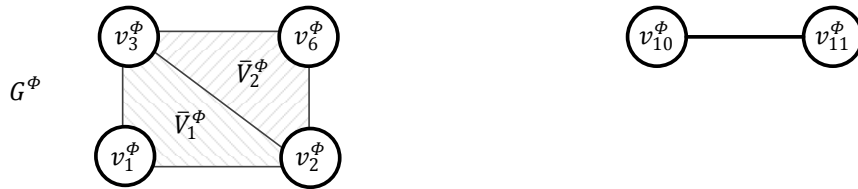
Figure 6.9: Clique search in the verification collision graph G^\Phi . In total, there are two maximal cliques exceeding the limit \tau = 2 : \bar{V}_1^\Phi and \bar{V}_2^\Phi . Both are comprised of three vertexes.
