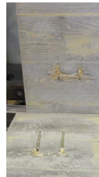
Figure 9: Push-Out-Test Result: Screw Type 1
