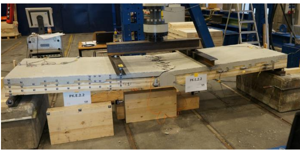
Figure 23: Four-point bending test on jointed CLT-TCC-elements
