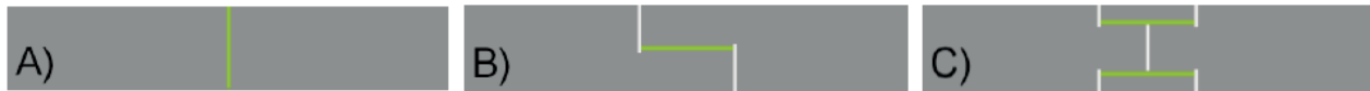
Fig. 3. Variations of in-plane CLT element connections with 10 mm compressed mineral wool stripes (in green), Kampmeier (2008) [4], Fig. 24.
