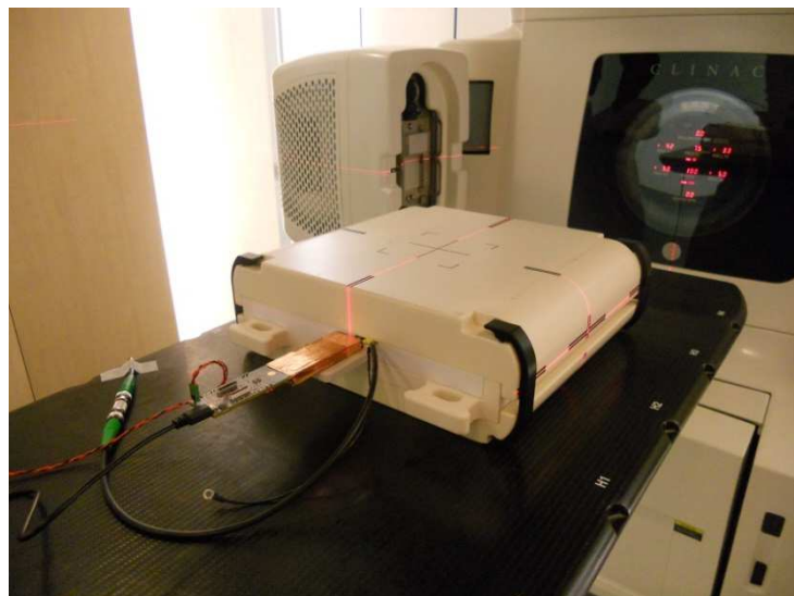
Figure 4.8. Detector array v2 inserted into the phantom and ready to be irradiated with the Trilogy® LINAC (Klinikum rechts der Isar) for patient plan verification.
