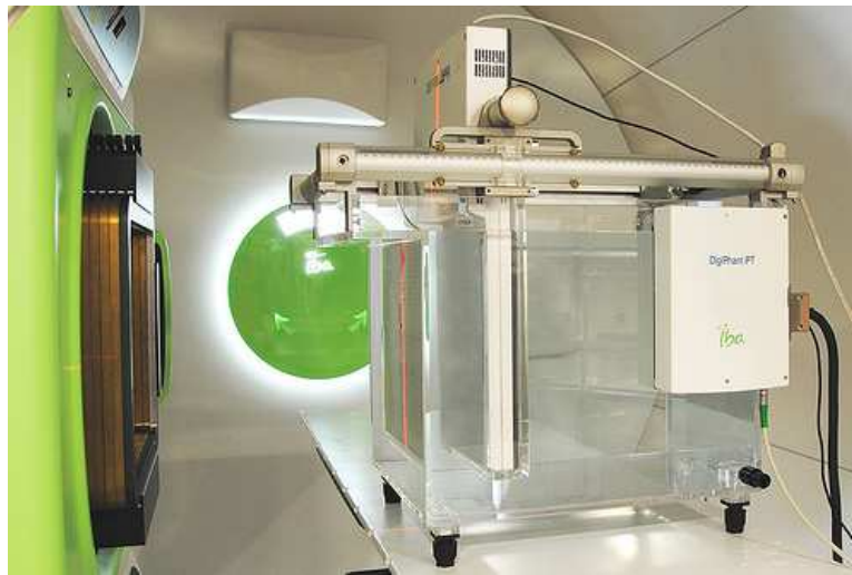
Figure 5.12. The 2D commercial ion chamber array MatriXX PT placed in the DigiPhant water tank (IBA Dosimetry GmbH, Schwarzenbruck, Germany). The detector can be shifted along the longitudinal beam axis to reproduce different depths of measurement in water.
