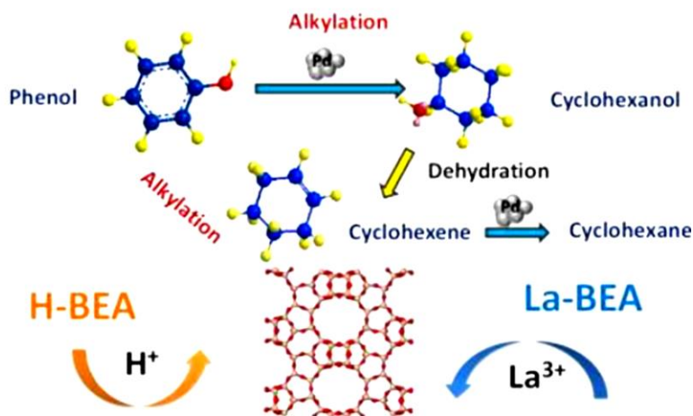
Figure 1.7. Phenol hydrodeoxygenation and hydroalkylation over Pd/C combined with zeolite H-BEA and La-BEA catalysts. [16]
