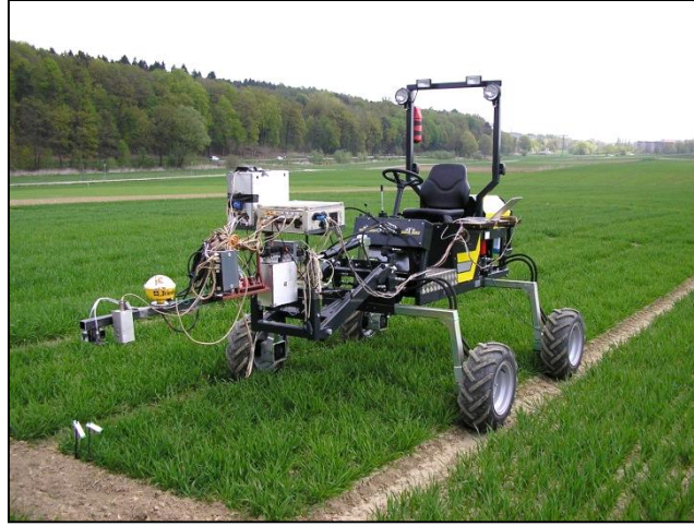
Figure 2: PhenoTrac4, carrying five passive and active spectral sensors.
