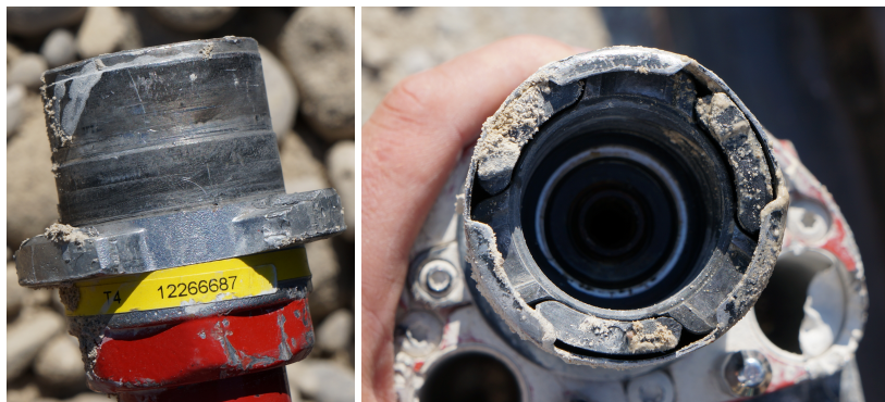
Dirts and dents at the interface between core bit and chuck
