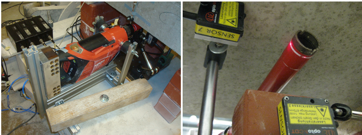
Figure 4.4: Measurement setup in which the machine is supported by a stand
