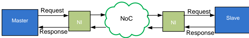
Figure 2.9.: Transactions representing interaction between master and slave for shared memory access
