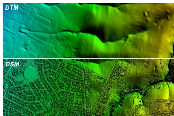
Figure 6.2 Digital Terrain Model vs Digital Surface Model over Adelaide, South Australia (Aerometrex, 2011)
