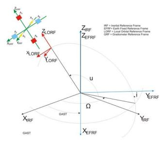
Figure 2: Definition of Reference Frames for GOCE Gradiometry
