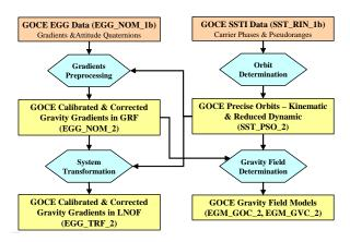
Figure 1: Simplified View of GOCE Level-2 Processing Sequence
