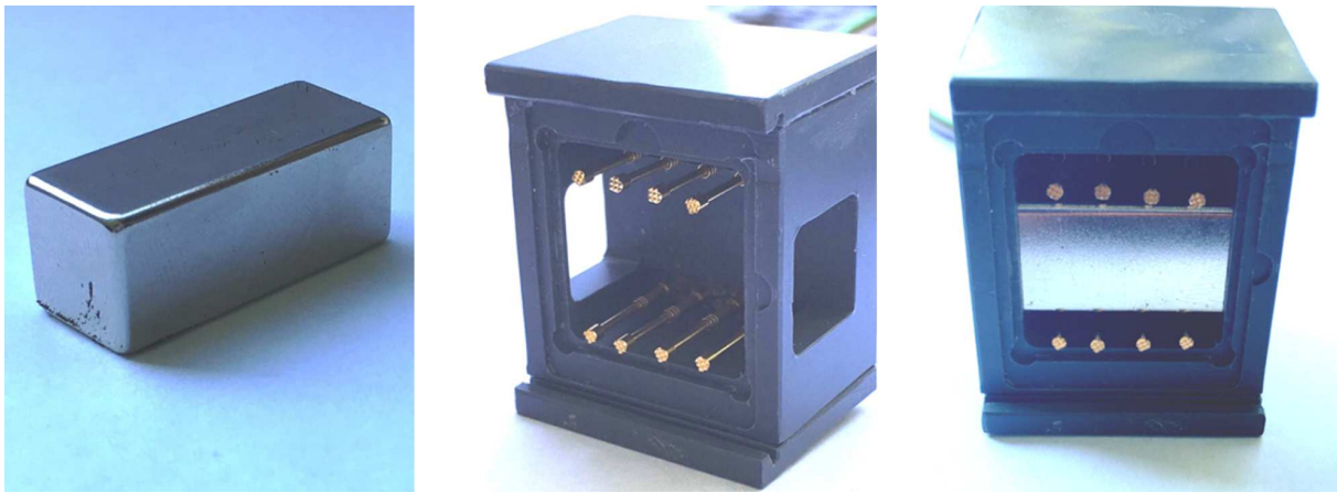
Figure A.5: a) Permanent cuboid neodym magnet used for the construction of the strong field-generating setup. b) Close-up of the modified empty PVC holder with larger distance between the test pin rows and two recesses for insertion of the neodym magnet. c) Front view of the assembled holder with the magnet and without the sample and the illumination mask mounted.
