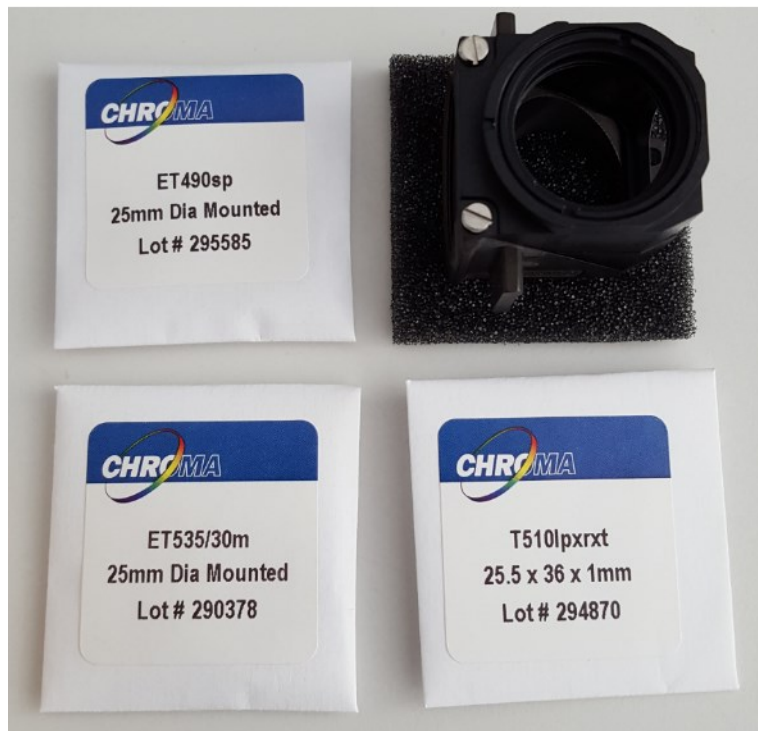
Figure.45 Overview of the excitation/emission system for the imaging of the roGFP2 cells at SNAKE and AIFIRA (upper). The system is based around dual excitation with individual excitation LEDs and a custom filter cube (lower) which filters the single emission wavelength back to the CCD. Filter cube components: Excitation filter: ET490SO; Emission filter ET 535/30; Dichroic mirror T510lpxrt.
