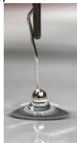
Figure 6-2: (A) Photograph of the setup used in this work and (B) the bead electrode in hanging meniscus configuration. Picture (A) is taken from reference [231].
