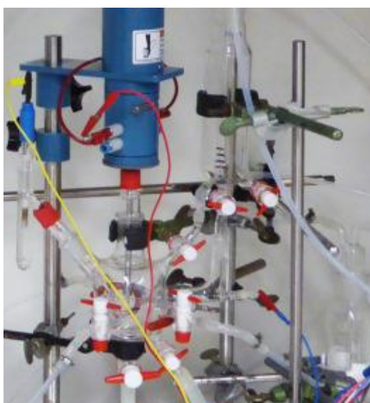
Figure 5-17: (A) Setup used in this work with installed rotating disk electrode. Taken from reference [231]. (B) Electrolyte flow towards a rotating electrode steadily supplying reactant-saturated electrolyte. Taken from reference [232].
