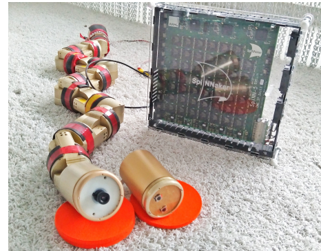
Fig. 1: Left: the snake-like robot equipped with stereo cameras/embedded dynamic vision sensor (eDVS) [5]. Right: The SpiNNaker board [6].
