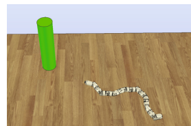
Fig. 2. The snake-like robot equipped with Dynamic Vision Sensor (DVS128)
