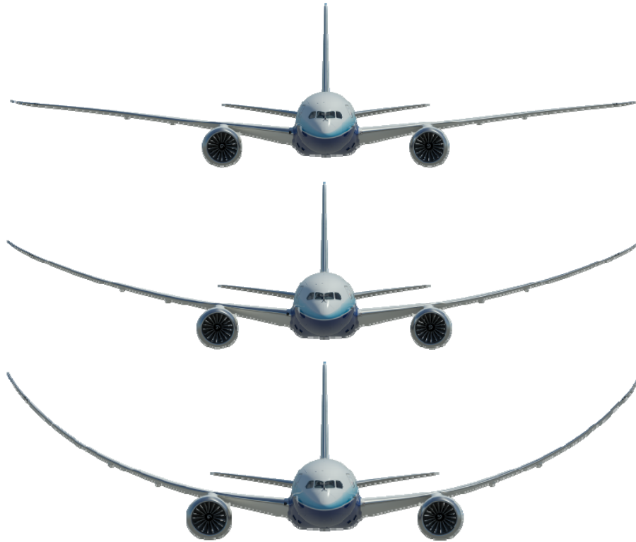
Figure 1.2: Wing displacements on ground (top), flight with 1 g (middle) and maximum load (bottom) of the Boeing 787 Dreamliner. (source: [Dod].)
