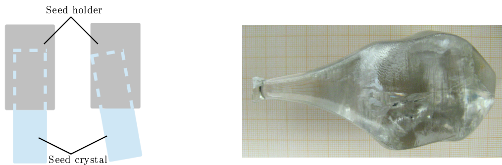
Figure B.1.: Seed crystal holding concept where the seed crystal sits too loosely within its holder and can easily be tilted (left). This tilt is comparable to a tilted orientation of the seed crystal. Due to growth anisotropies in the different directions within the crystal, the result is an asymmetric raw crystal (right). As an additional factor, also the crystal weight plays a role which finally leads to huge stresses and cracks inside the crystal ingot.
