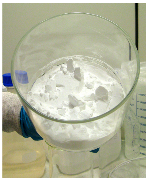
Figure 5.6.: Cleaned \text{CaCO}_3 powder after TOPO extraction and back-transformation via a precipitation reaction with the help of a \text{Na}_2\text{CO}_3 solution (compare equation 5.1).
