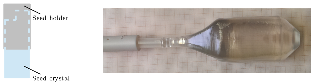
Figure B.2.: Seed crystal holding concept where the seed crystal is fixed by a step within the holder (left). As this concept is not rotationally symmetric, the resulting raw crystal (right) shows a slight asymmetry.
