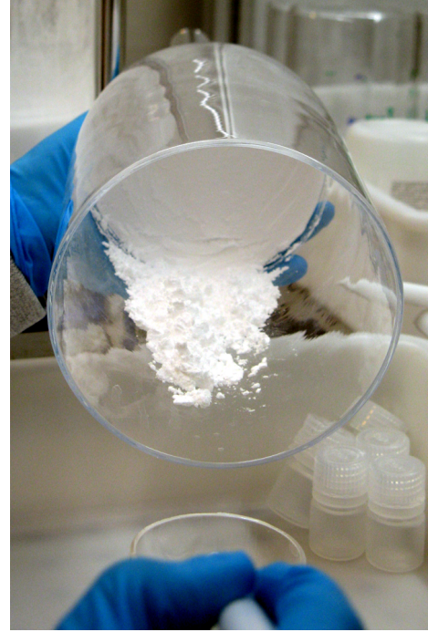
Figure 5.10.: CaWO 4 powder produced via the precipitation reaction including all purification steps described in sections 5.3.2 (version 2), 5.3.3, and 5.3.4. The resulting product is a fine and homogeneously white powder.
