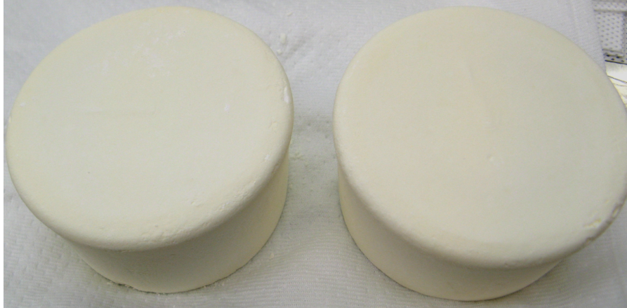
Figure B.6.: \text{CaWO}_4 "stones" after production via the solid state reaction from purified \text{CaCO}_3 powder (version 1). To be able to clean the material from sodium and potassium contaminations, the material had to be heated up to \sim 600^\circ\text{C} and plunged into cold (supra-pure) water. This method made the \text{CaWO}_4 porous enough to be pulverized with an agate mortar.
