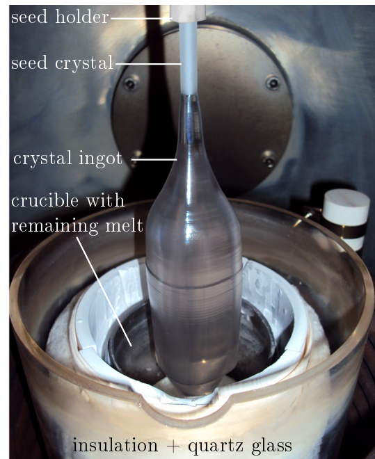
Figure 3.6.: \text{CaWO}_4 crystal ingot hanging down from its seed crystal and holder after growth in the Czochralski furnace (here without after-heater, shown in figure 3.7). The remaining melt is solidified at the bottom of the crucible which is surrounded by insulation to minimize heat losses during growth.
