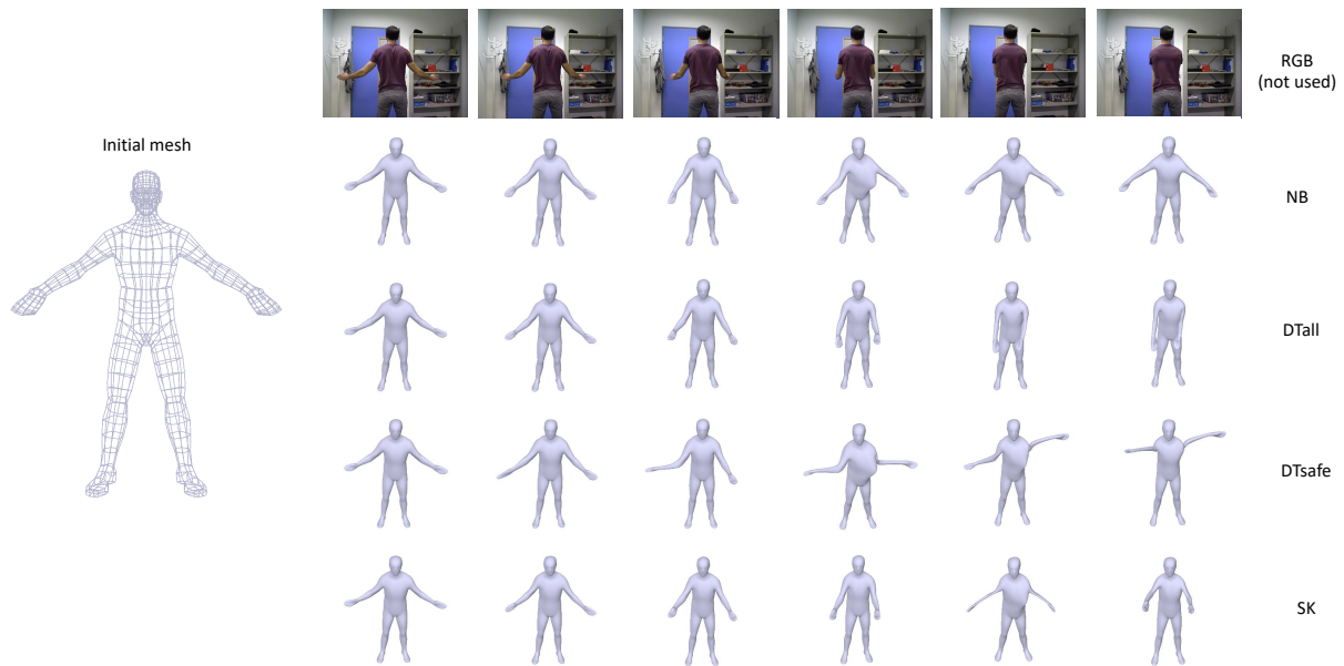
Figure 5.9: Results after running the optimization problem to align a given initial mesh of a person with geometric data associated to different postures. The first tested images (left columns) observe a person whose posture is close to the initial mesh while the person’s posture in the the last ones (right columns) is considerably different from that of the initial mesh.
