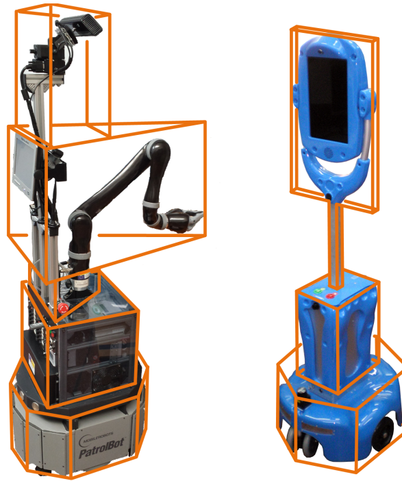
Figure 6.5: Example of 3D geometric models of the Giraff robot (right) and Rhodon (left).
