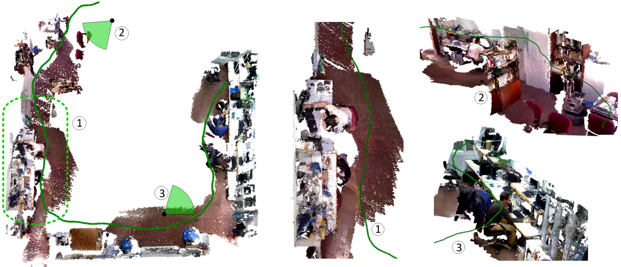
Figure 3.5: Three-dimensional map of our lab generated with an RGB-D camera from DIFODO motion estimates. An overall top view is shown (left) together with some local views: a detailed top view (1) and two perspective views (2 and 3). The camera trajectory is depicted with a green continuous line.
