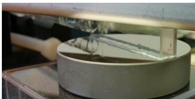
Figure 2.5.12: Spectroscopy cell being glued to one of the two nickel-molybdenum coated quartz electrodes. The width of the remaining optical windows of the cell is 1 cm.
