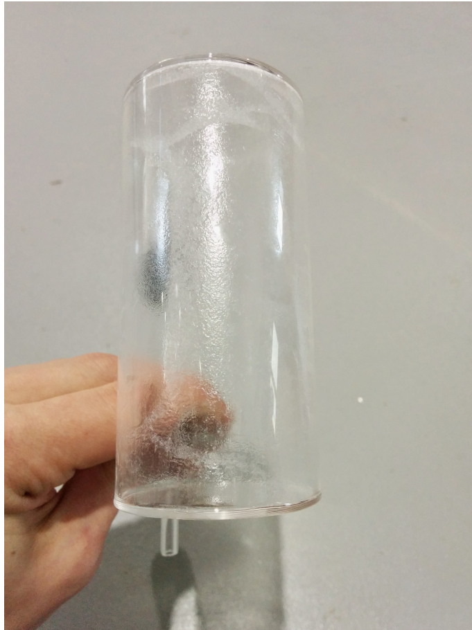
Figure 3.5.2: Side view of the all-quartz cell that was used as precession cell in the shielding factor measurement. The empty cell was provided by Timothy E. Chupp from the University of Michigan. The quartz was visibly coated with paraffin.
