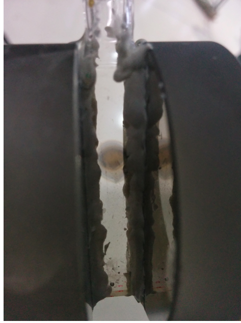
Figure 2.2.1: A first prototype cell for the Stark shift measurement (2.5.3). This cell had a vacuum leak and a second layer of glue was added to improve the vacuum. The cell that was used for the measurement was built with much less glue. The dark spots in the middle are likely to be oxidized mercury.
