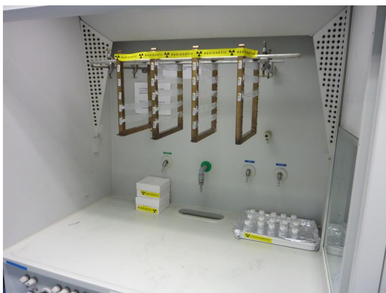
Fig. 2.6.2: Fume hood with exposed SPMD on frames and reference samples in glasses.
