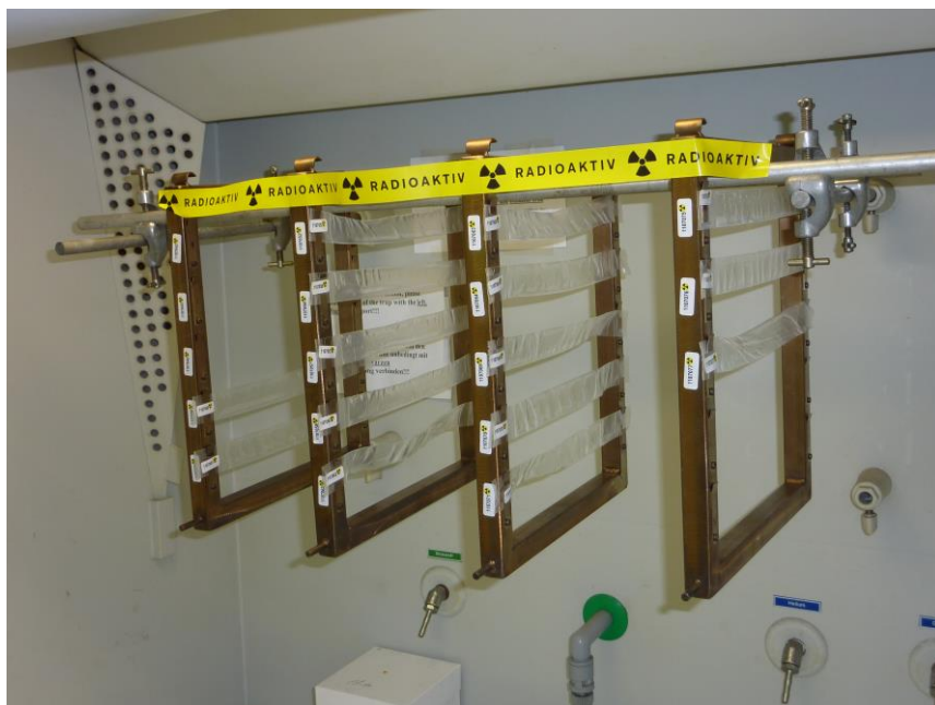
Fig. 2.6.1: Close up view of SPMD on frames.
