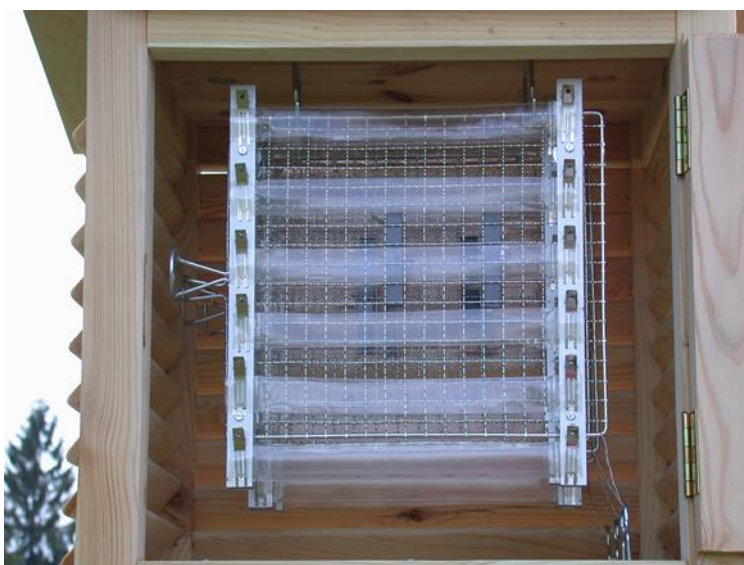
Fig.2.5.1: The VO expose into Stevenson screen box
