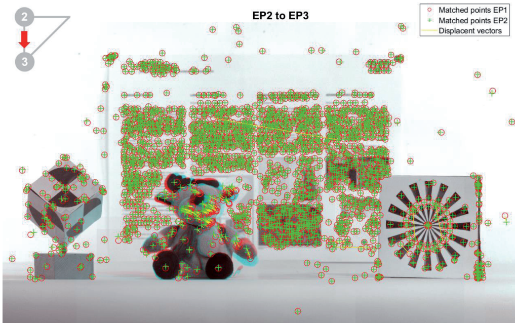
Fig. 5 Result of a SIFT matching of two different epochs/toy positions
