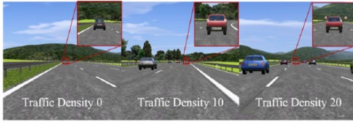
Figure 2. Examples of the takeover situations from the ego vehicle's view at the moment of the takeover request. Inset zooms in on the stopped vehicle, representing the system limit.
