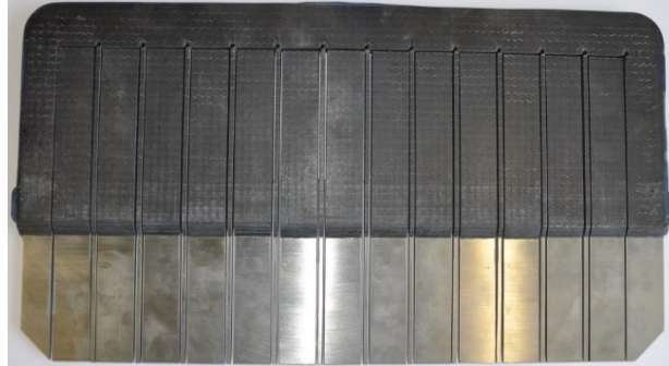
Figure 4-11: Image of a trimmed hybrid composite/metal panel of joint design 1
