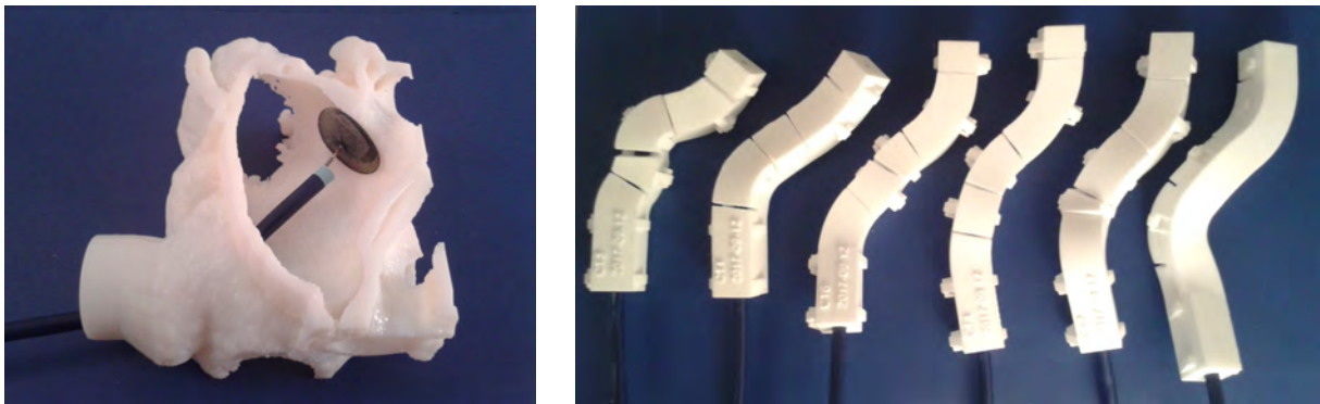
Figure 91 The catheters are introduced into the additively manufactured models and the implant is deployed in the LAA (left). The image on the right shows the six bending forms for the catheter shape with four bends.
