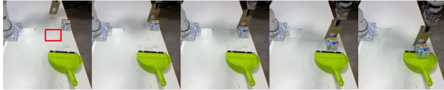
Fig. 10: Motion execution for an object not used during the training. The red rectangle represents the bounding box of the initial trash positions in the collected dataset. The object is placed outside the range of training data for evaluating the extrapolation performance.
