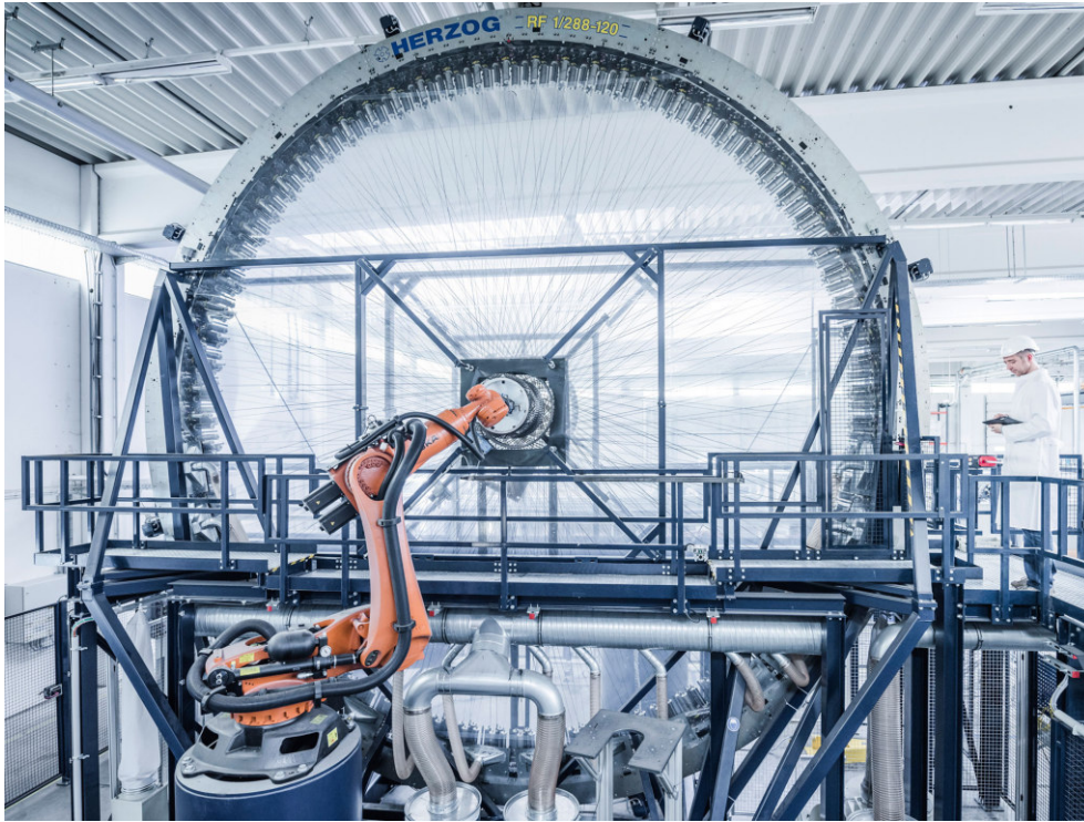
Fig. 2.1: Radial braiding machine with 288 carriers for CFRP wheel production
