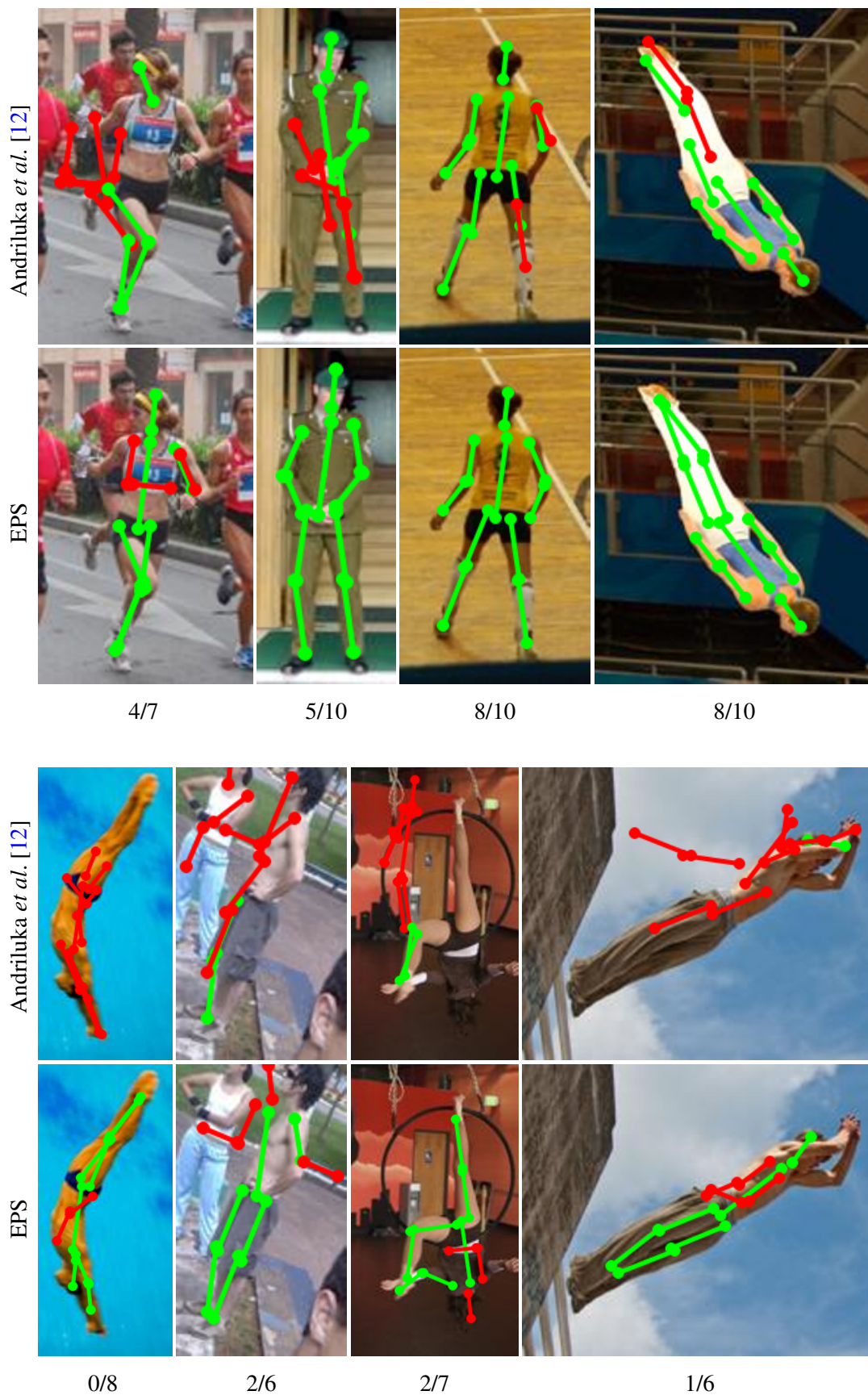
Figure 2.7: Pose estimation qualitative comparison. Example images from LSP dataset, with poses estimated by Andriluka et al. [12] versus our complete 2D model (EPS). The numbers under images show the number of correct parts by [12]/EPS.
