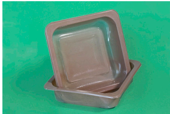
Figure 2. Thermoformed trays (144 mm × 144 mm × 40 mm) containing gallic acid as the O 2 scavenger.
