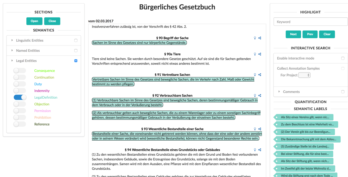
Figure 3.2.: View of an automatically annotated German law (left: annotation type selection using check boxes; middle: annotated and highlighted text; right: labels visualizing the annotations separately).
