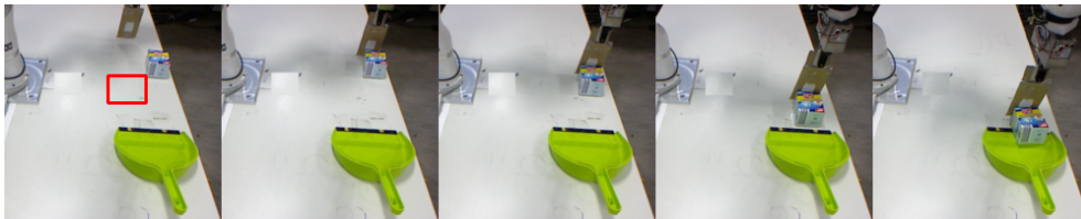
Figure 4.9.: Motion execution for an object not used during the training. The red rectangle represents the bounding box of the initial trash positions in the collected dataset. The object is placed outside the range of training data for evaluating the extrapolation performance.
