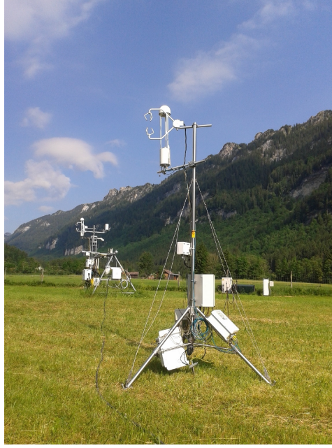
Figure 12: Photograph of the mobile mast in the front and the permanent eddy covariance mast in the background.
