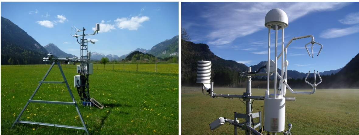
Figure 11: Left: Photograph of the measurement tower in Graswang towards the west; Right: Photograph towards the east with the eddy covariance system consisting of a sonic anemometer (CSAT3), and two gas analyzers (LI7700 and LI7500); for more details see Section 3.4.
