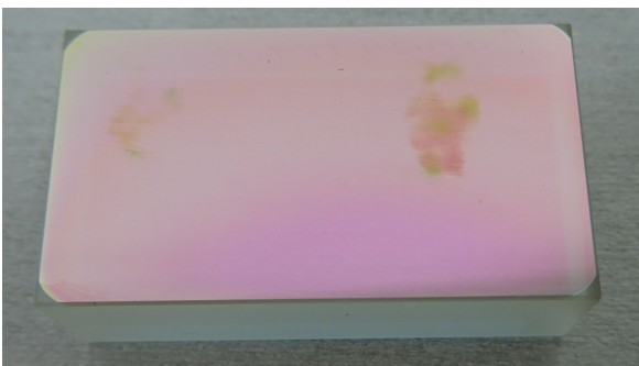
Figure 7.2.: Example of a contaminated DCM surface. The stains are located at the former beam positions.
