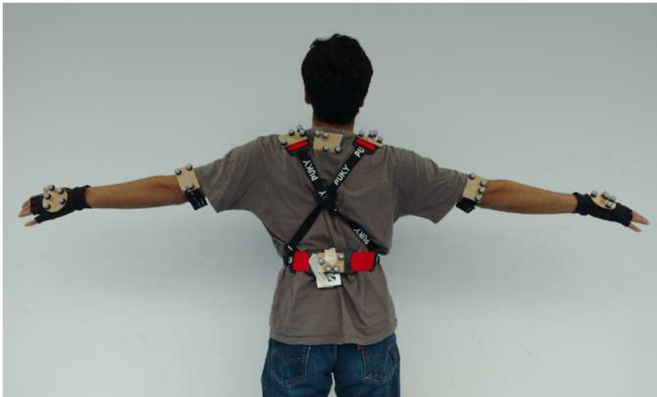
Figure 1.4: Marker cluster positions on a human subject
