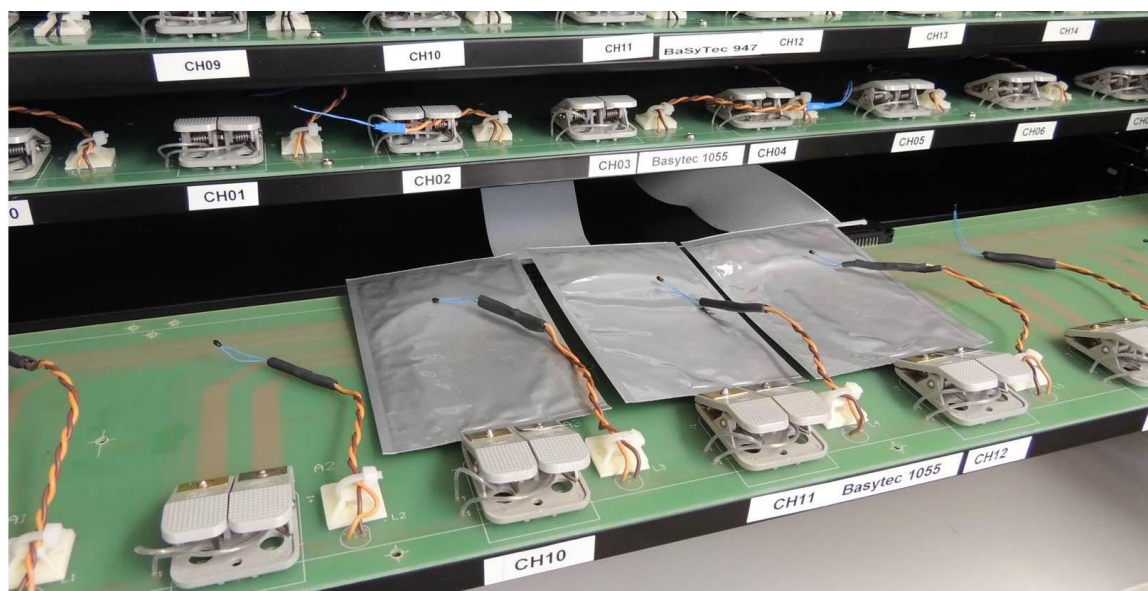
Figure 12: Prepared full-cells mounted on a BaSyTec rack. Each full-cell is equipped with a temperature sensor on top as a safety measure in case of battery failure.
