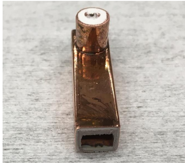
Figure 42: ABS-Core with electroplated copper
