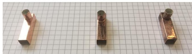
Figure 43: Copper shells with 50 μm, 100 μm and 150 μm copper
