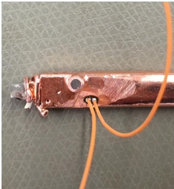
Figure 41: Soldered wires on test body (left) and batch 6 (right) after electroplating process
