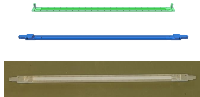
Figure 29: 4 th generation LC-cavity (top: ‘lid’, middle: ‘body’, bottom: glued LC-cavity)
