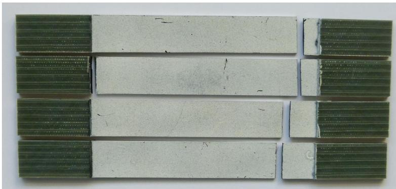
**Fig. 5-23** Quasi-static specimen failure mode of DIN tests.
