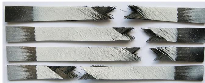
**Fig. 6-4** Quasi-static specimen failure mode of DIN tests.
