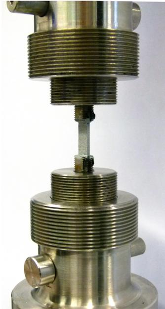
**Fig. 5-17** Quasi-static tensile test setup.
