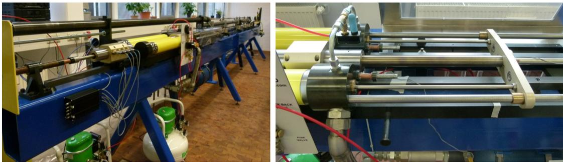
Fig. 3-11 SHTB (left) with a sliding carriage connected to pulling rods that guides the striker-bar (right).
