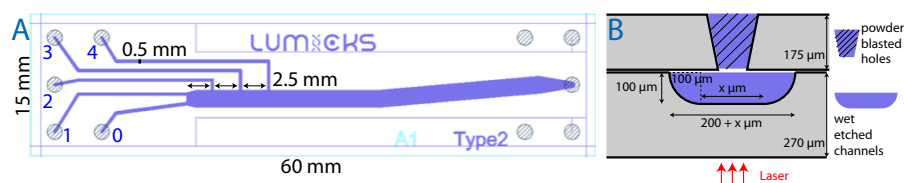
Figure 2.7: (A) First design of microfluidic chip. The five different channels (purple) are connected to the inlet holes (shaded circles). They are then combined and connected to the outlet hole. (B) Etching geometry of microfluidic chip channels and inlet holes.
