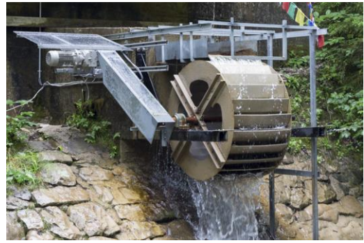
Fig. 1. Prototype overshot waterwheel at Söllbach, Germany.
