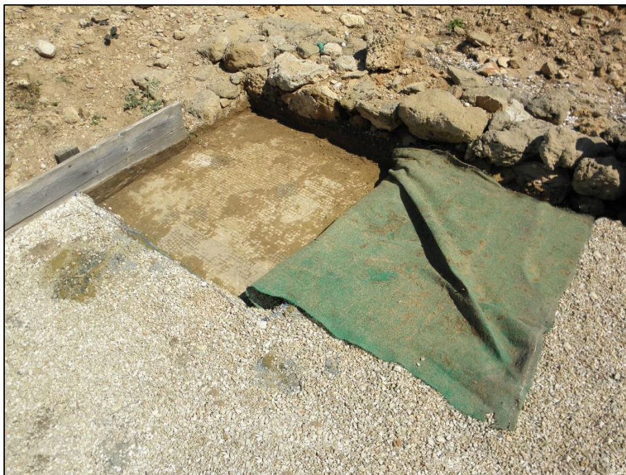
Fig. 26 An inspection of the effects of a long-term, maintained reburial at the World Heritage Site of Nea Paphos, Cyprus in which a synthetic fabric was used
