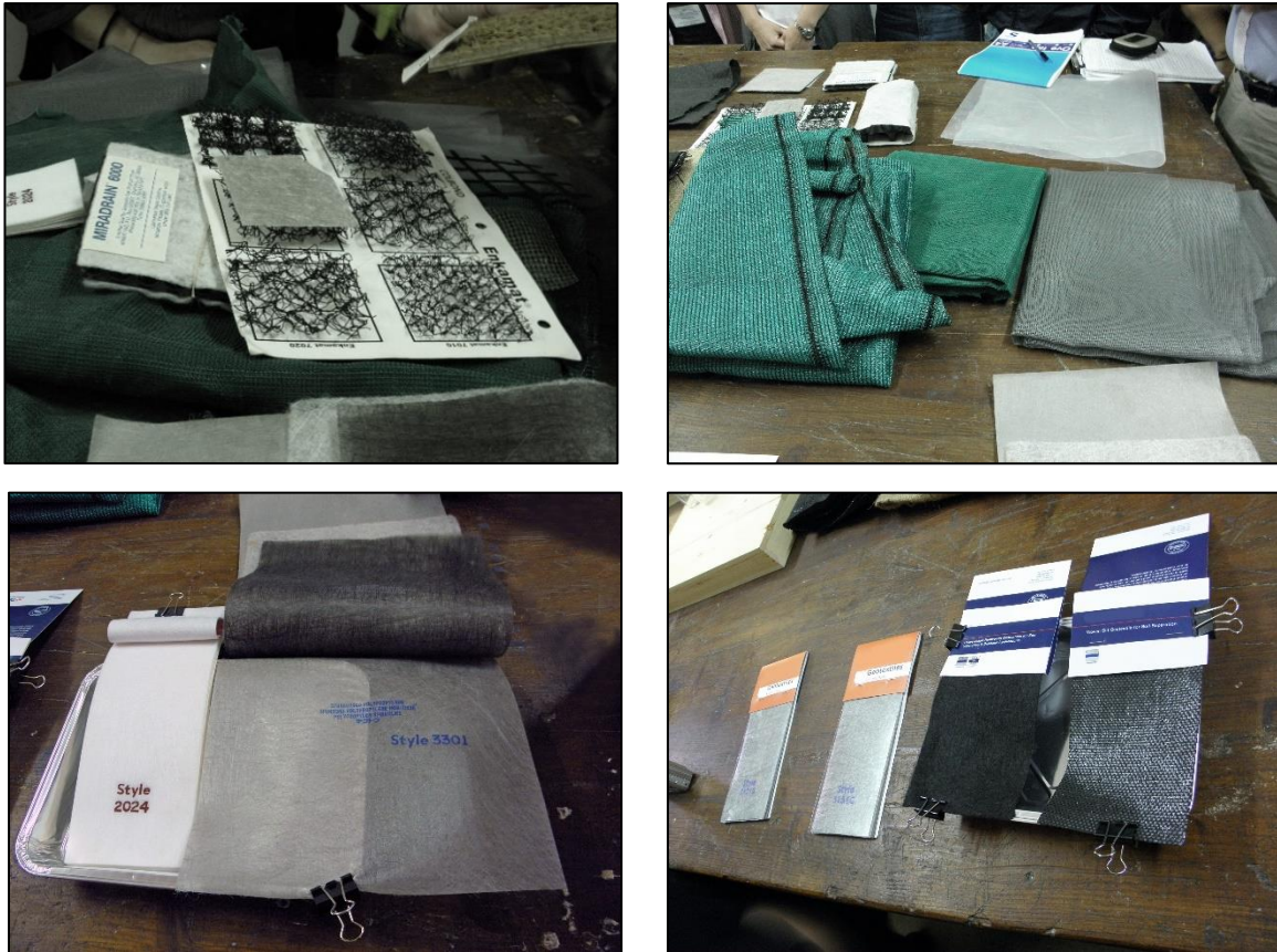
Fig. 21 – 24 Temporary and permanent erosion control nets (upper right), synthetic fabrics (upper left) and geotextiles (lower left and right) used in slope stabilisation and site reburial
