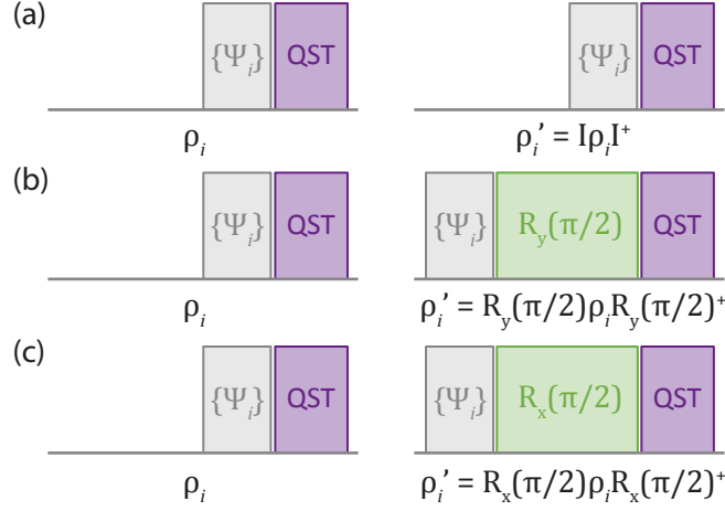
Figure 2.32: Schematic pulse protocols for QPT. In the first step, QST is performed on a set of independent states \{\Psi_i\} . Afterwards, QST is performed on the same set of states, to which a quantum operator is applied. This can be (a) the identity operator, (b) a rotation of \pi/2 about the y -axis and (c) a rotation of \pi/2 about the x -axis. For this kind of measurement, an IQ -modulated setup (cf. Fig. 2.24) is necessary in order to control the qubit phase.
