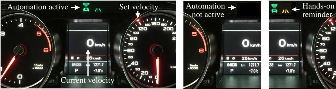
Figure 4.5: Visual feedback in the instrument cluster, referring to Cramer et al. (2018)
