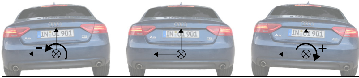
Figure 2.4: Roll motion of the test vehicle with a negative (left in the figure) and a positive (right in the figure) roll angle compared to the horizontal position of the vehicle chassis (middle in the figure), referring to Cramer et al. (2018); Cramer, Lange, et al. (2017)
