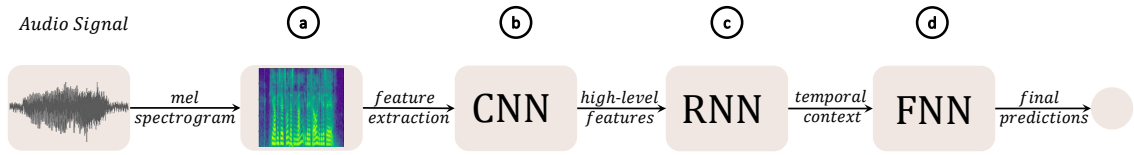
Figure 7.1: Illustration of the proposed CRNN approach composed of convolutional and recurrent neural networks for feature extraction and a feed forward network to generate the final predictions. A detailed account of the procedure is given in Section 7.2.
