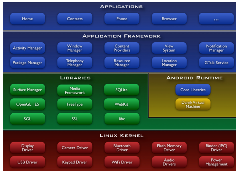
Figure 2.1: Android's Software Architecture [14]
