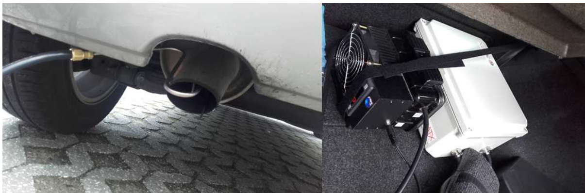
Figure 36. On-board emissions measurements
