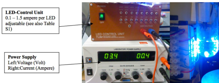
Left: TUM LED Control Unit. Right: Irradiation of catalytic mixture with 450 nm LEDs.
