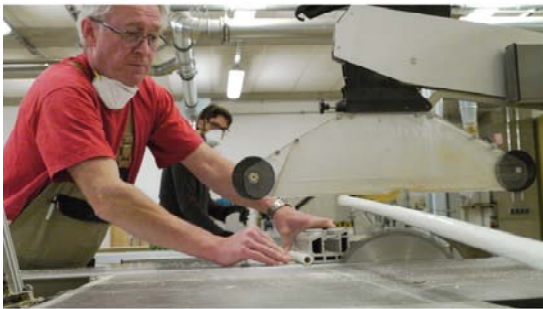
Figure 12: Cutting the GRP tubes
