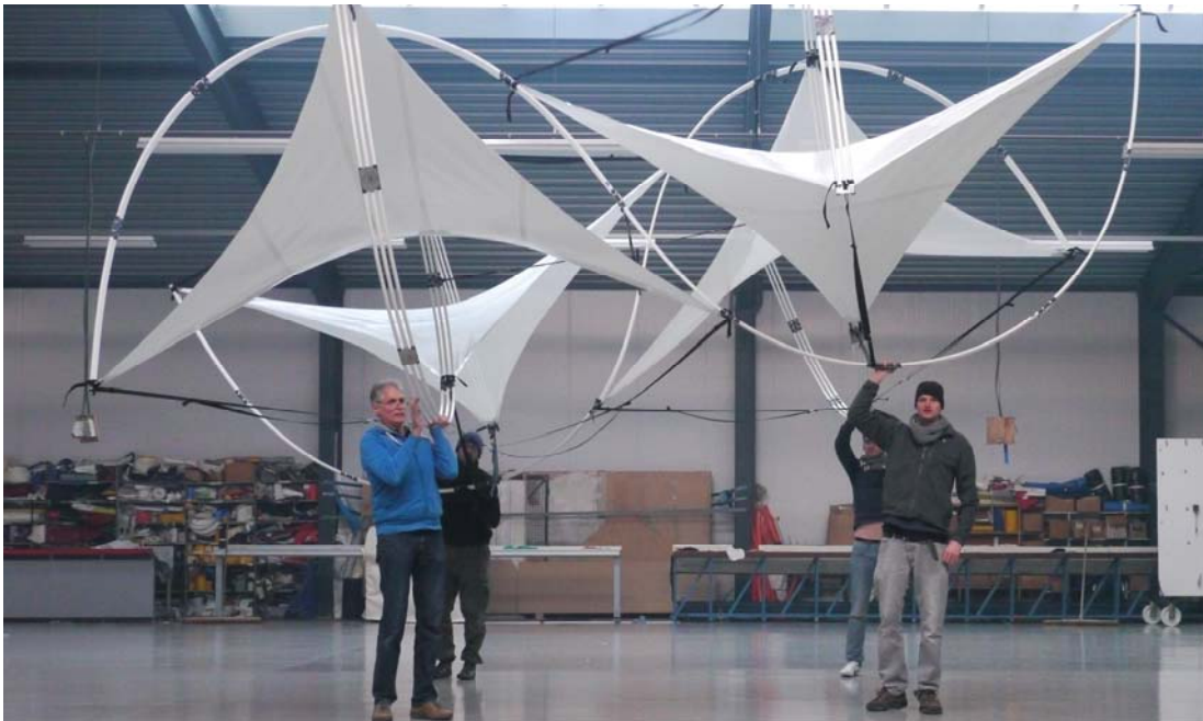
Figure 17: Assembly test of the "bending-activated tensegrity"-structure
