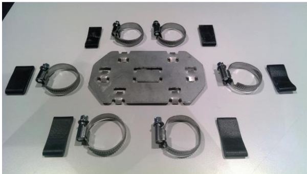
Figure10: Coupling - aluminum plate with hose clamps and rubber interlayer
