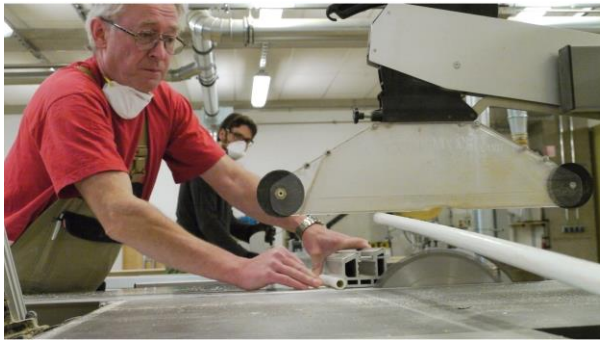
Figure 8: Cutting the GRP tubes
