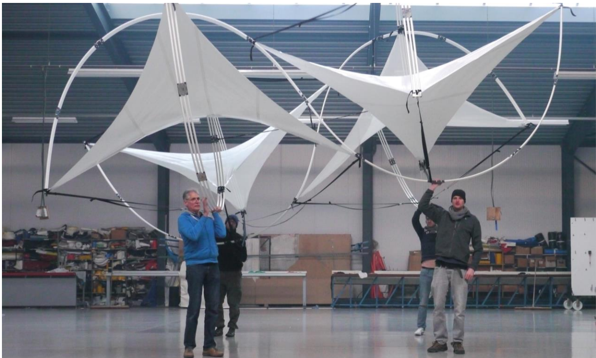
Figure 13: Assembly test of the 'bending-activated tensegrity'- structure
