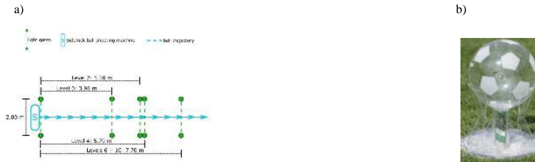
Fig. 1. (a) hardware setup for test measurements; (b) a glass model of the ball's transmitter and inductive charger.
