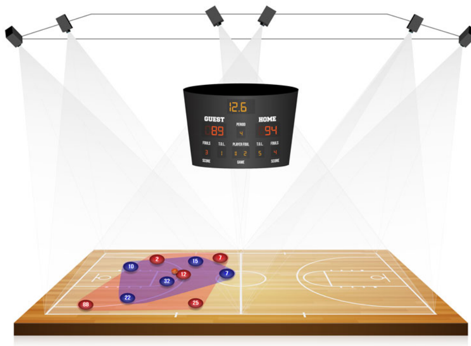
Figure 2.1: “Moving dots” are the result of the application of player tracking systems. This example shows the camera-based Stats SportVU tracking system for basketball. Image taken from Stats (2019).
