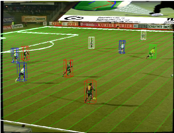
(a) Result of player detection and labeling steps for tracking football players. Bounding boxes, coloured by team identity, are drawn around players. Figure taken from Beetz et al. (2006) .
