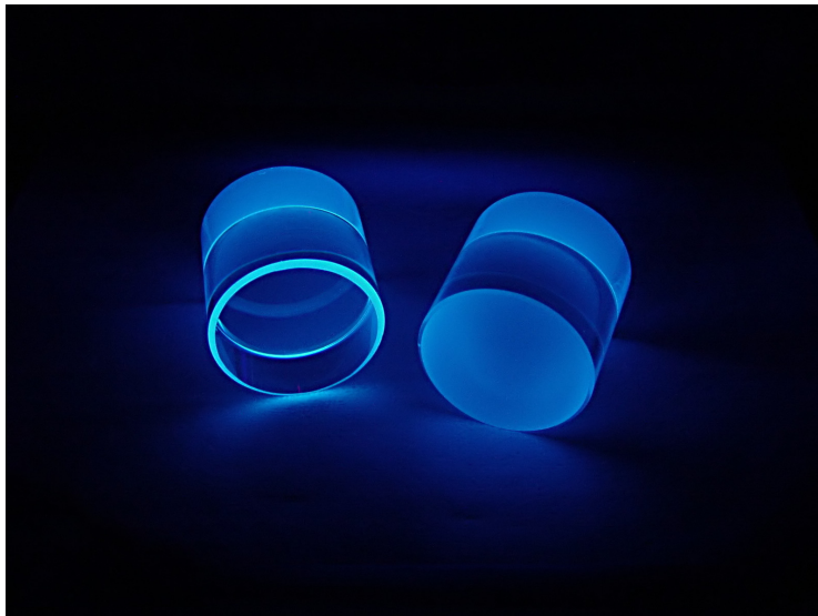
Abbildung 2.4: Photograph of scintillating \text{CaWO}_4 crystals under UV light excitation. The blue emission of the scintillation spectrum peaks at (420 \pm 30) \text{ nm}/(2.9 \pm 0.2) \text{ eV} .
