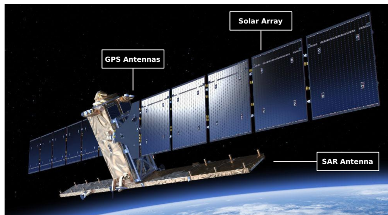
Fig. 2.4: Artist's view of the Sentinel-1A spacecraft, indicating selected equipment. Courtesy: ESA
